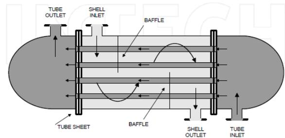
**Figure 2.2 Heat exchanger with one passes at the tube side**
