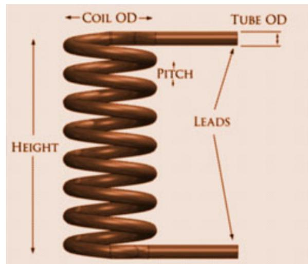
Fig. 3.4 Coil type tube
