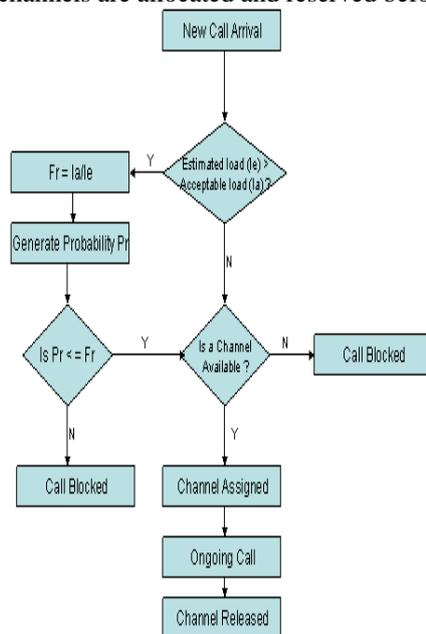
**Figure 2.3.1.1: Flow Chart for CAC Algorithm**
