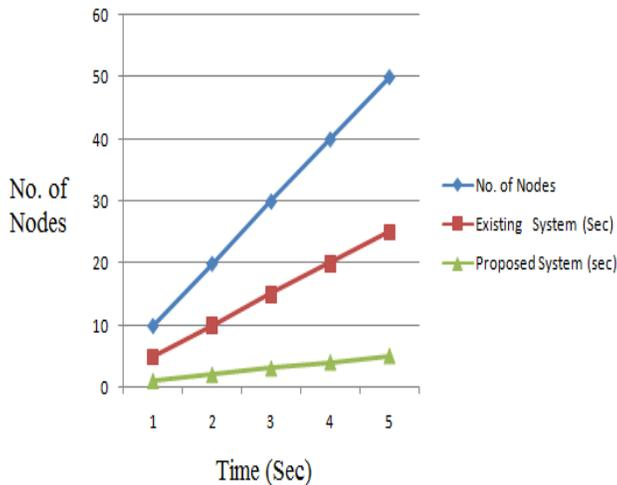
Figure 6 :- Comparison Between Latency Period of Data Sending in existing & proposed system.
