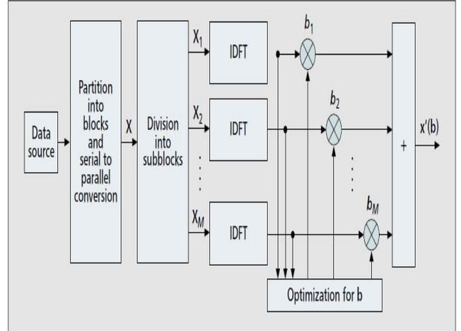
Fig 3. A block diagram of the PTS technique.
