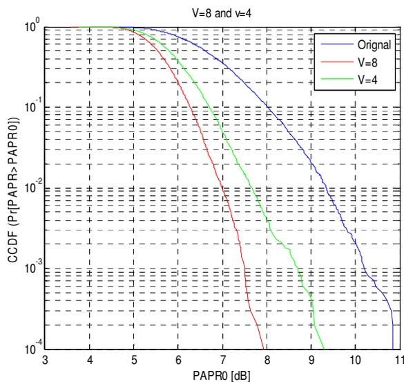
Fig 4. CCDF of PAPR by PTS for various V
