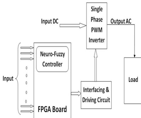
**Figure 3.1: Diagrammatic representation of the proposed work**
