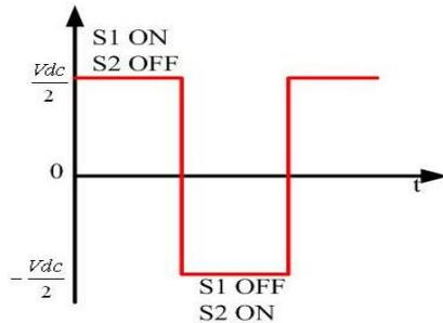
**Figure 3.1.2: Inverter Output**
