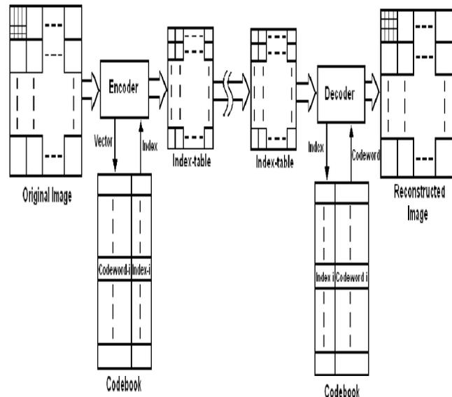
The flowchart of LBG Algorithm is as given under,(7)
