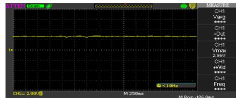
We wave a hand in front once and we can see the output changing during that time. Note the fast changing wave at first and then getting steady as we stop waving hand in front.
