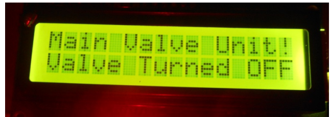
Figure 5(f): When all tanks are filled turn of the motor or main valve
