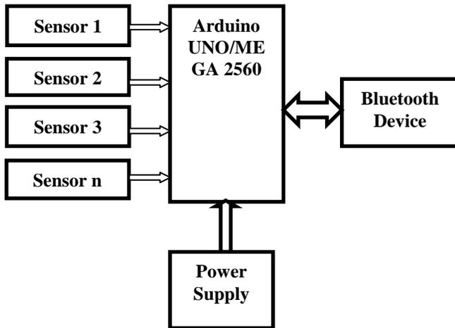
Fig.c] Wireless Sensor Node
