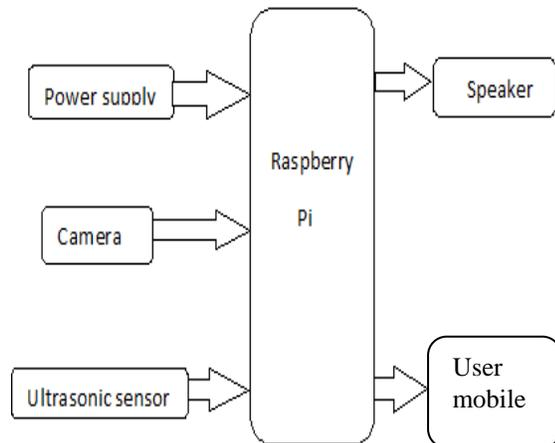
**Fig i]: Functional Block Diagram of the Project**
