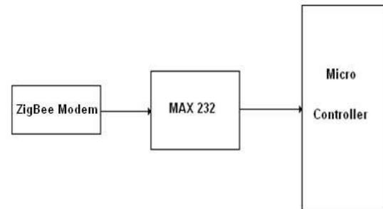
**Fig of:3.3 Interfacing Zigbee to Microcontroller**
