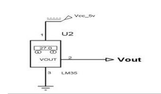
**Fig of: 3.1 Interfacing Circuit**
