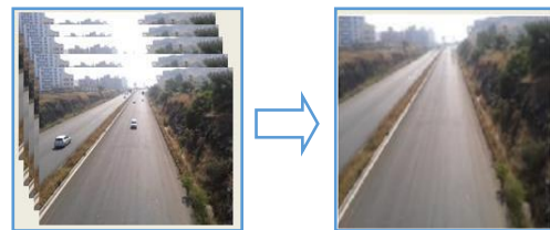
Fig III.2.1.1 Background model using averaging frames[2]
