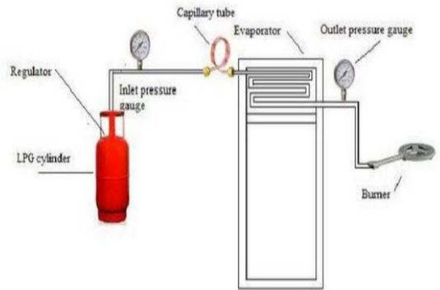
**Fig. 3** Setup of LPG refrigeration system
