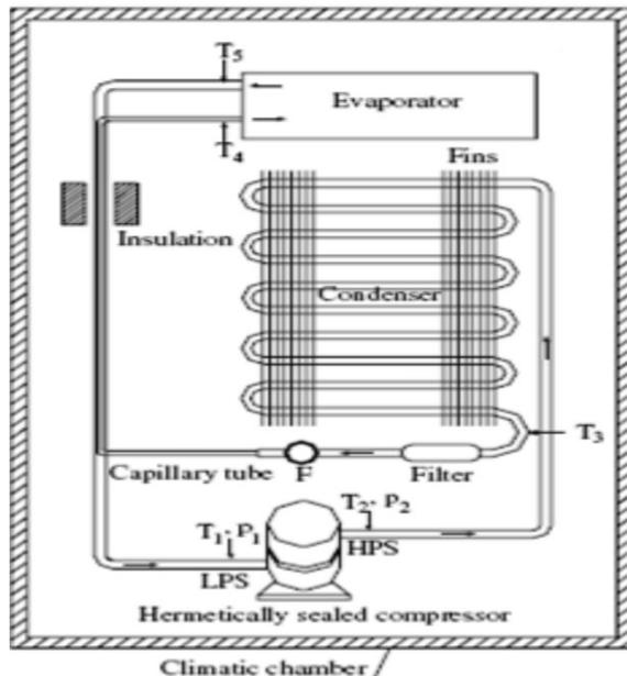
**Fig.4** Schematic Diagram of Equipment in Fridge Circuit
