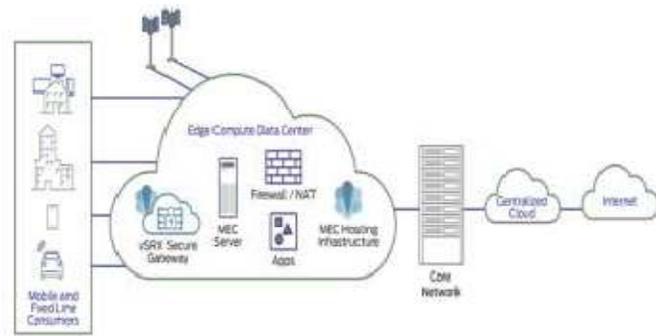
Fig.2 Architecture of Multi-Access Edge Computing (MEC)
