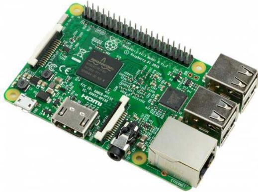
**Fig.2: Raspberry pi model B**
