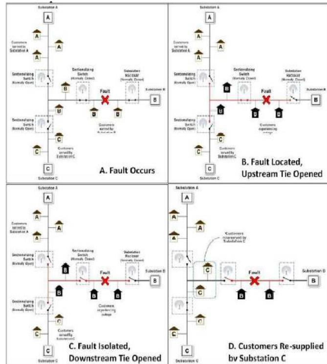
Figure 3:- Schematics illustrating FLISR Operations.
