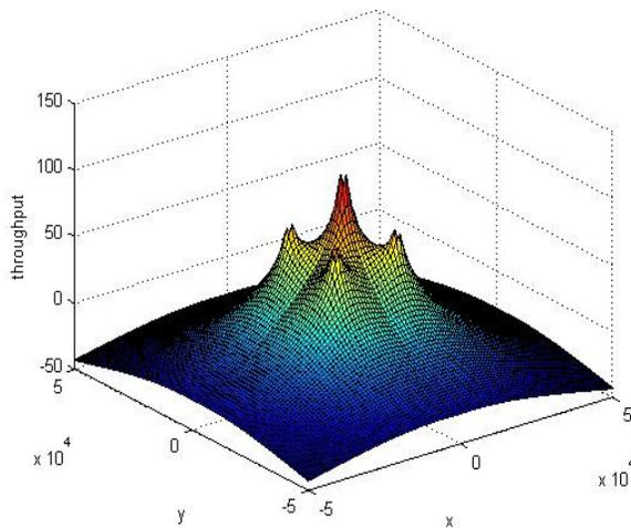
Fig. 4. The throughput for normal relay with downlink transmission  $x$ =transmitter,  $y$ =receiver,  $z$ =Throughput
