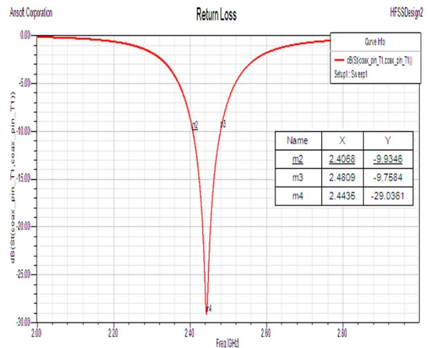
Fig.1. Return Loss of -29.03 dB at 2.45GHz.
