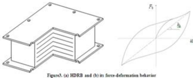
Figure3. (a) HDRB and (b) its force-deformation behavior
