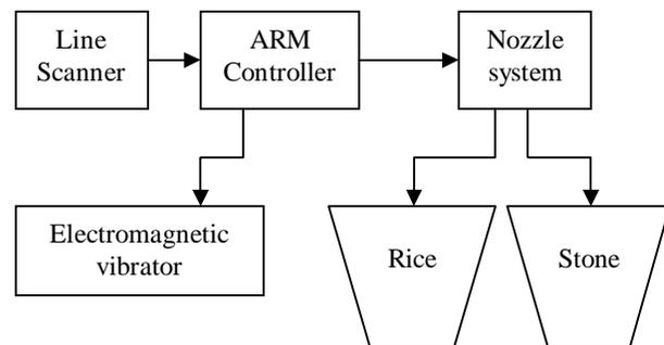
**Fig1:** Block diagram of rice cleaning machine
