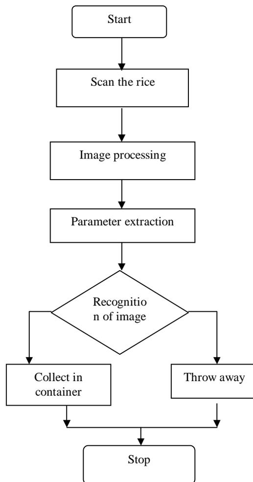
**Fig 3:** Flow chart of the sorting procedure
