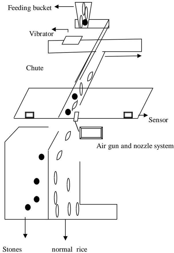
**Fig 2:** structure of rice cleaning machine
