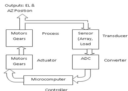
**Figure 1 Closed Loop Control System**
