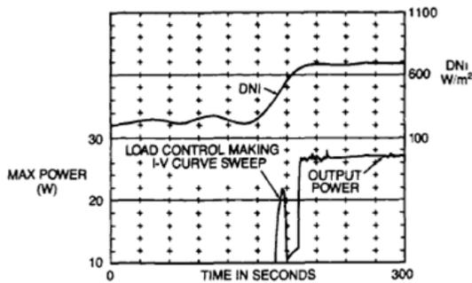
**Figure 5 Tracking and Control operation when cloud passes**
