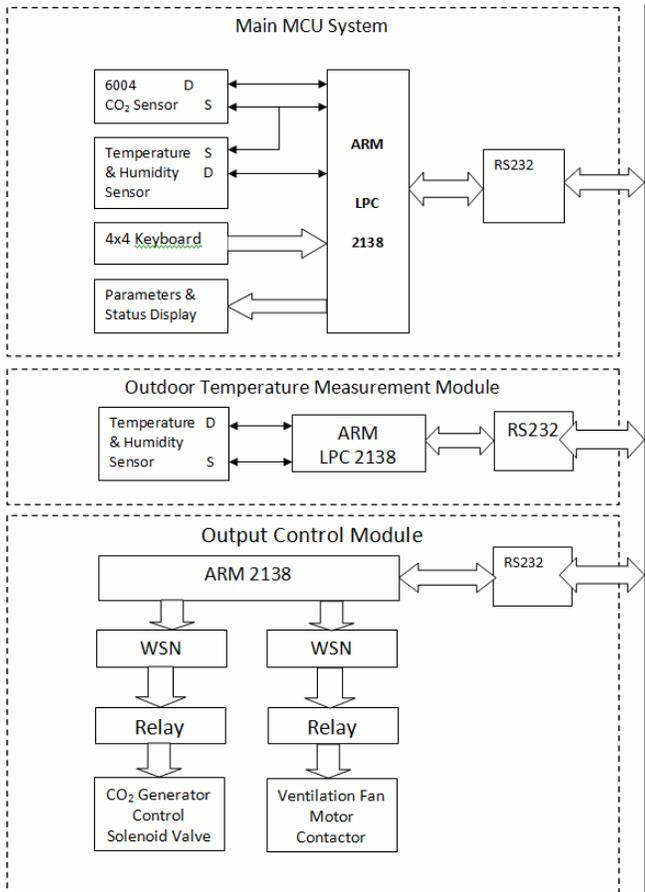
Figure1. Agricultural greenhouse carbon dioxide measurement and Control system hardware architecture
