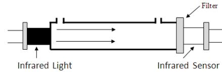
Figure 2. NDIR schematic diagram of infrared gas analysis
