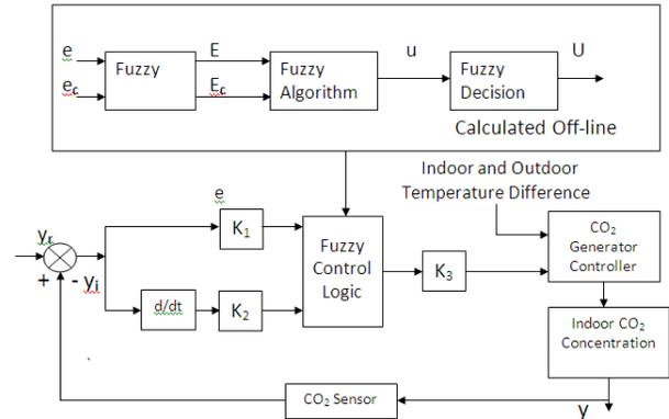
Figure 3. Schematic diagram of carbon dioxide concentration fuzzy
