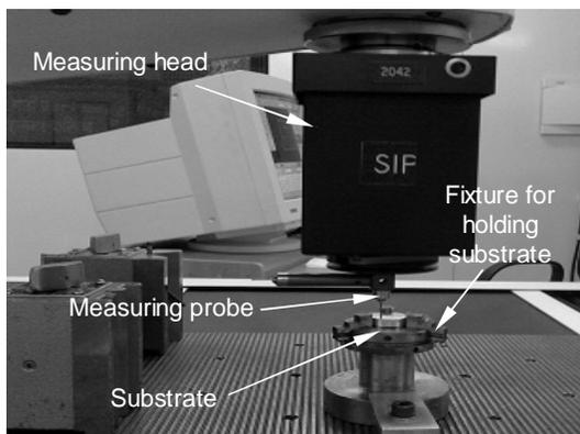
Fig. 2 Universal Measuring Machine (UMM)
