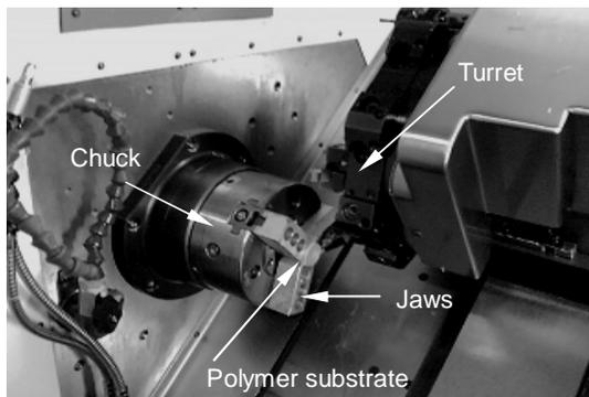
Fig. 1 Close view of set up of CNC turning operation
