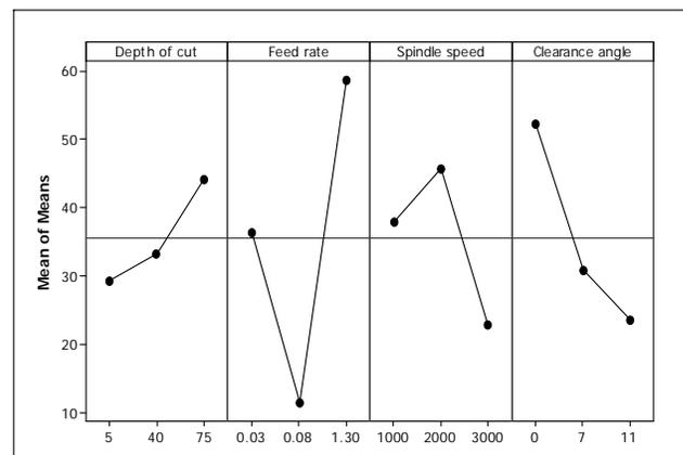
Fig. 4 Main effects plots for flatness in CNC turning of Polypropylene
