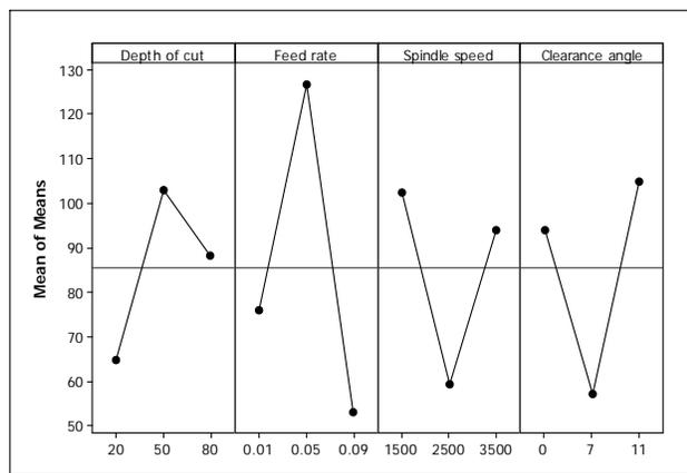
Fig. 3 Main effects plots for flatness in CNC turning of Nylon
