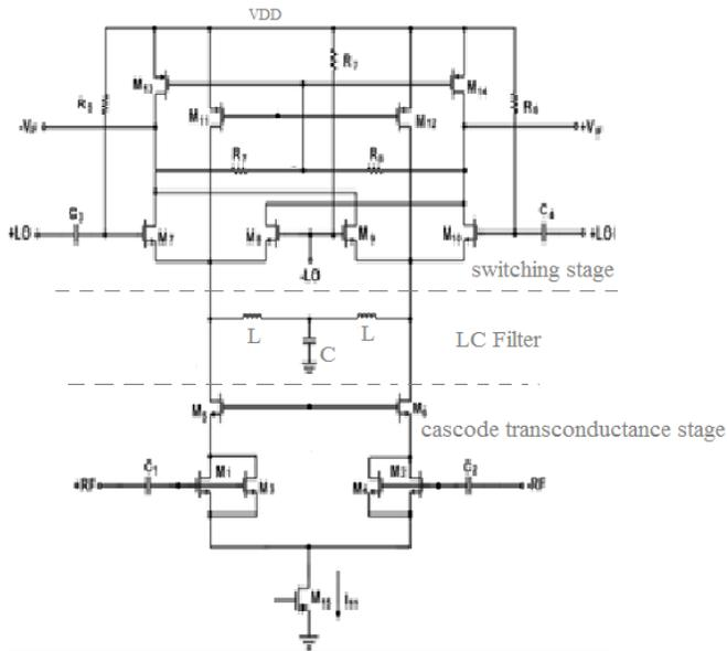
Figure 3 Double balanced Gilbert mixer with LC filter and current bleeding technique
