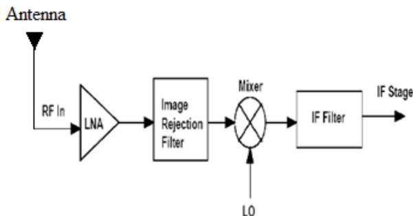
Figure 1 RF receiver front-end
